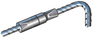
The P14 style couplers are designed to splice two curved, bent or straight bars, when neither bar can be rotated and where the on-going bar is free to move in its axial direction. Typical applications for these couplers are for the splicing of pile cages. The P14 position coupler can be separated in two pieces for application against form work. Reducers / Transitions available upon request.
