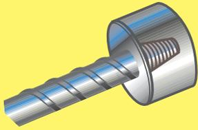
The LENTON TERMINATOR provides an alternative to hooked rebar, or an anchor or stop nut for rebar passing through a pile plank or structural steel element. The front face of the coupler is generously designed to carry the full tension load of the rebar when the anchor is bearing against concrete or structural steel.
