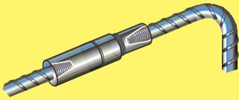
The P9 and P14 style couplers are designed to splice two curved, bent or straight bars, when neither bar can be rotated and where the on-going bar is free to move in its axial direction. Typical applications for these couplers are for the splicing of pile cages.
