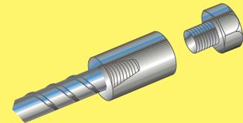
LENTON bolt couplers provide a full strength joint between a reinforcing bar and a standard metric bolt. The coupler may be used for load-carrying steel structures bolted to concrete foundations, columns or walls, such as pylon bases, fixing crane rails, and fixings for heavy pipe work and walkways.
