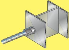
LENTON weldable couplers provide a quick and easy solution for connecting reinforcing bar to structural steel sections or plates. Similar to the standard coupler, the weldable coupler is internally taper threaded on one end, with the other end prepared for welding.
