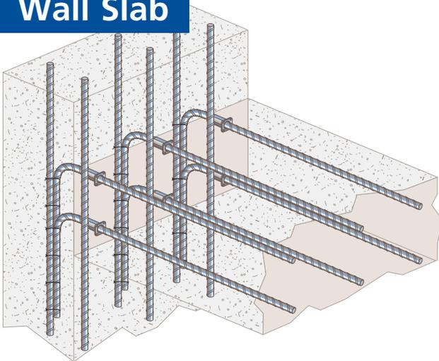
LENTON FORM SAVERS for wall/slab or wall/beam connections eliminate the need to penetrate the formwork. Indispensable when using sliding or climbing formwork.
