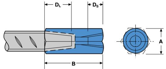
LENTON transition couplers are designed to splice different diameter bars where one bar can be rotated and the bar is not restricted in its axial direction.
