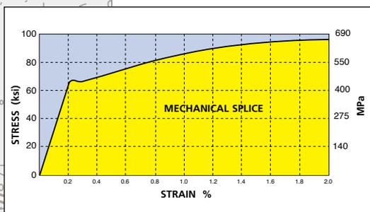
*Mechanical splicing provides significantly higher strength by design than lap splicing.*
