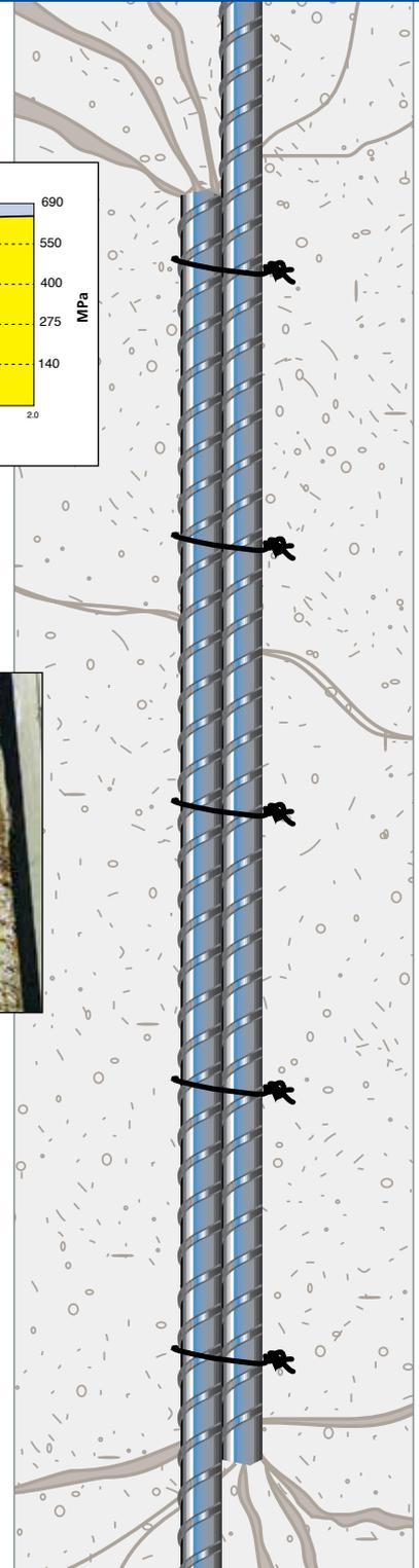
*Lap splices depend on concrete for strength, and therefore lack structural integrity and continuity in concrete construction.*
