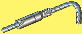
P8 and P13 style couplers are designed to quickly splice two curved, bent, or straight bars, when neither bar can be rotated, and where the ongoing bar is restricted in its axial direction. Typical applications for these couplers are for the splicing of prefabricated cages.
