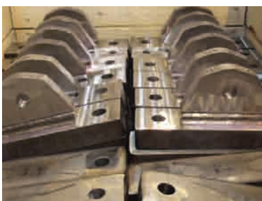
Tunnel Ceiling Suspension Systems
